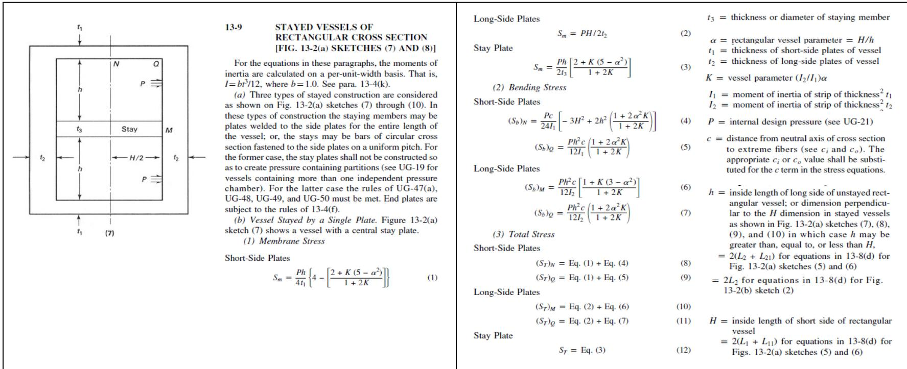
A-M Figure 4 – Stress Analysis Excerpt for Stayed Rectangular Tank (316L SS)
