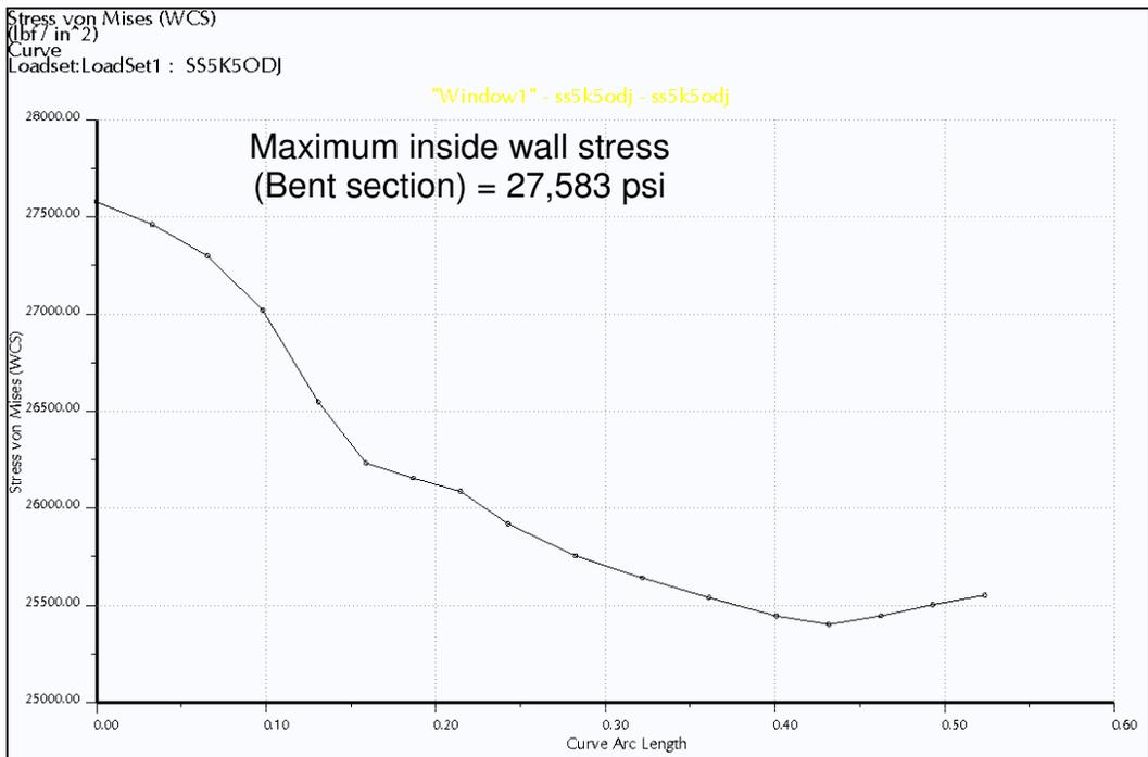
A-I Figure 12 – Stress vs Arc Length (Inside Rim of Bent End, 0.5” OD)
