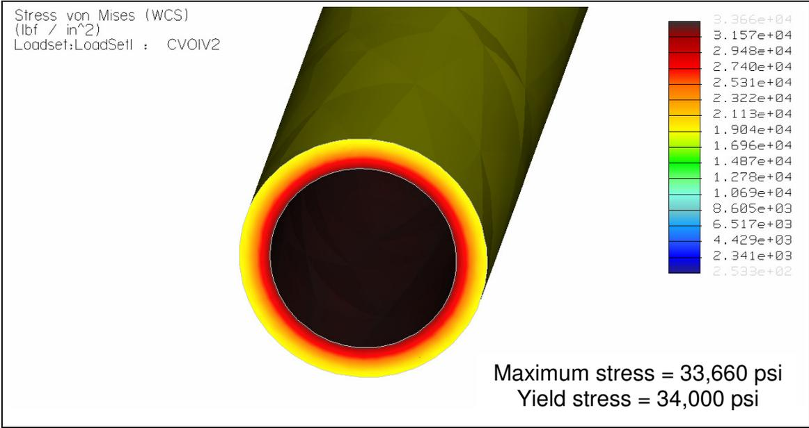
**A-H Figure 3 – 316L SS Cylinder Fringe Plot – Transverse Cut Close-Up**
