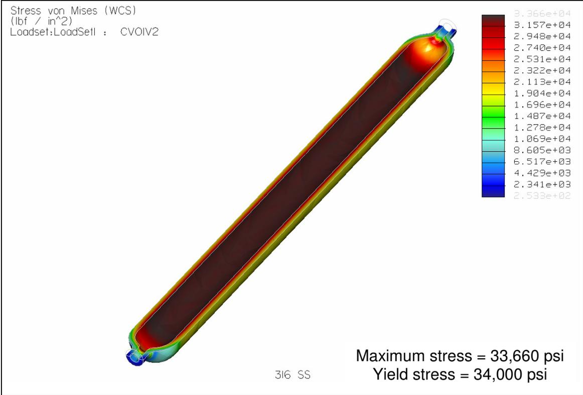
**A-H Figure 4 – 316L SS Cylinder Fringe Plot – Longitudinal Cut**
