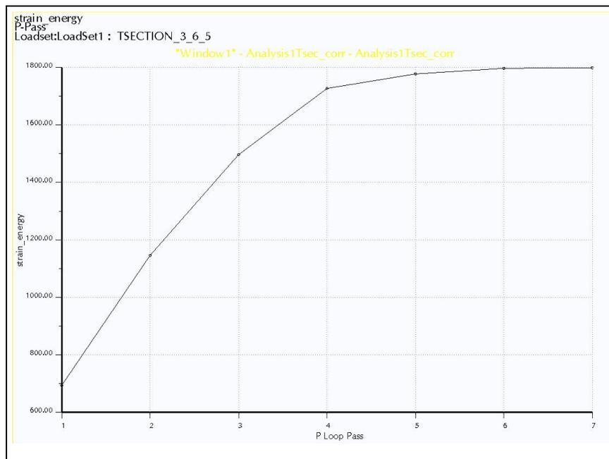
**A-J Figure 32 – 4130 Q&T Hydrostatic T-Section 10% Convergence Plot**
