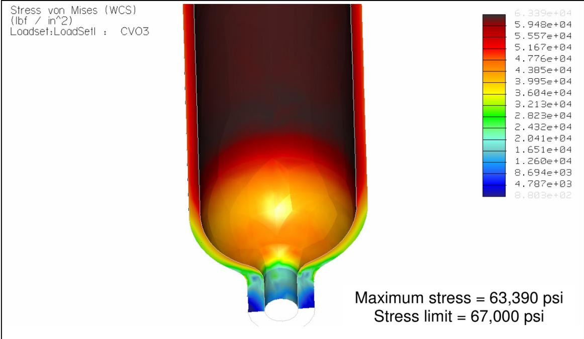
**A-H Figure 11 – 4130 Q&T Cylinder Fringe Plot – Longitudinal Cut Close-Up**
