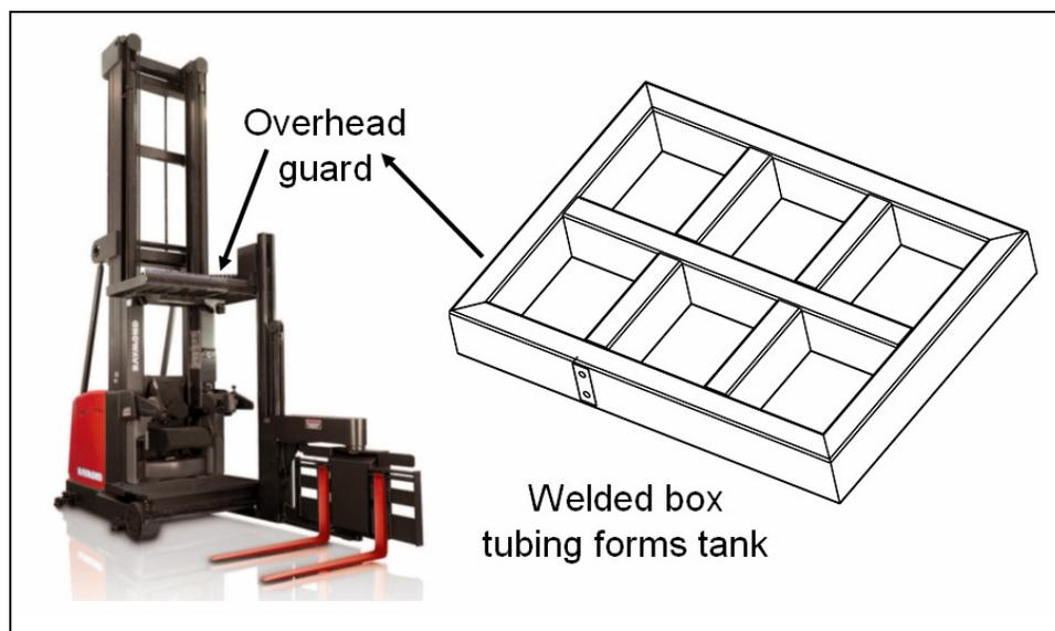
Figure 24 – Overhead Guard Becomes Tank
