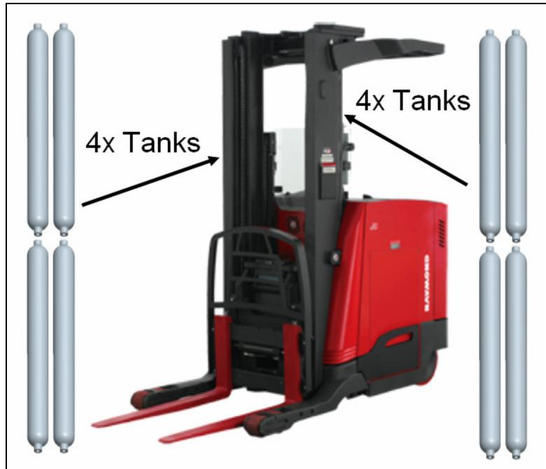
**Figure 9 – Revised Mast-Mounted Configuration**
