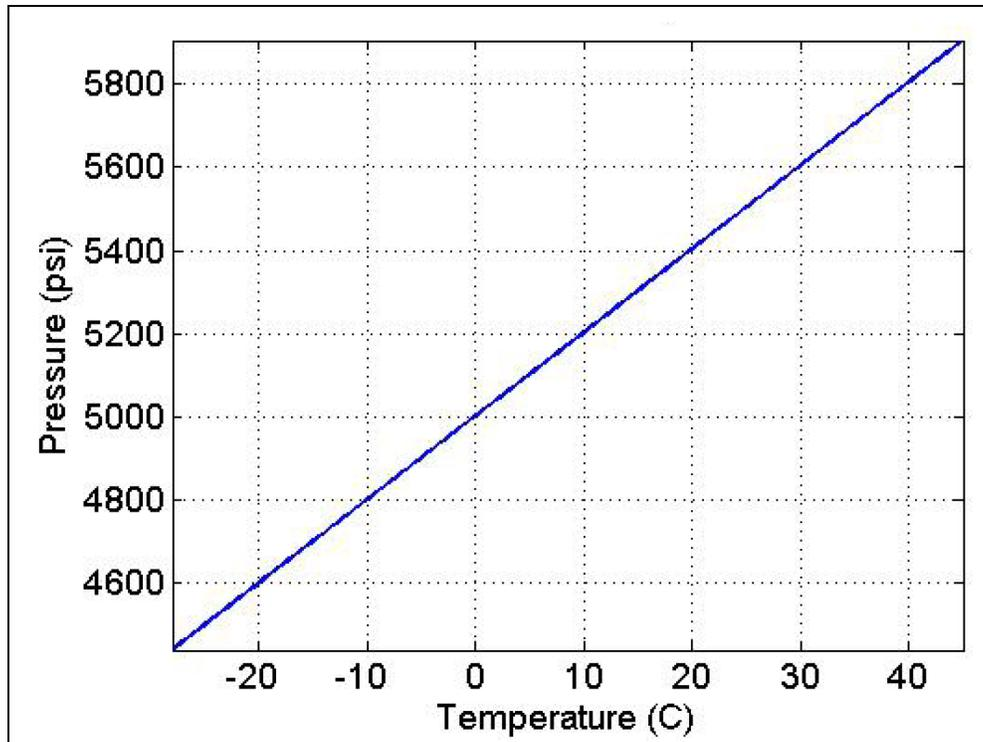
**Figure 3 – Temperature vs H<sub>2</sub> Tank Pressure**
