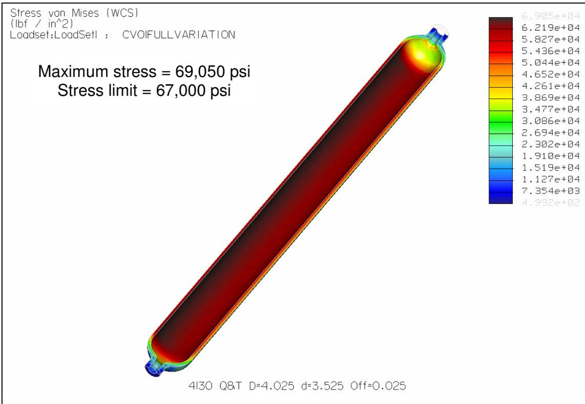
**A-H Figure 19 – 4130 Q&T Cylinder Fringe Plot – Case 3 Variation**
