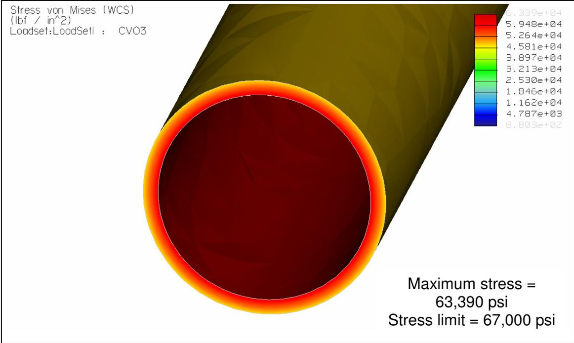
A-H Figure 9 – 4130 Q&T Cylinder Fringe Plot – Transverse Cut Close-Up
