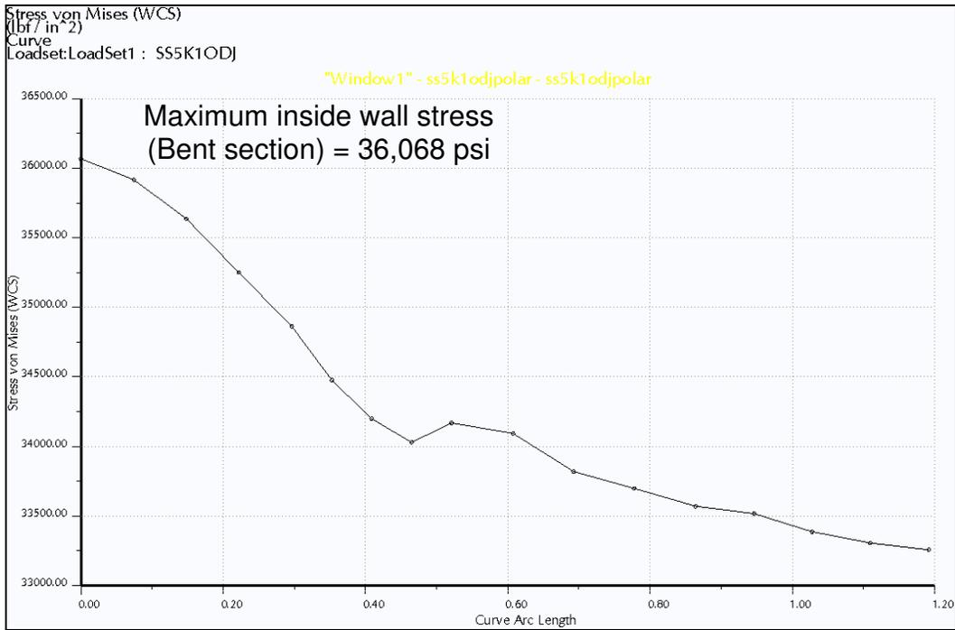
A-I Figure 9 – Stress vs Arc Length (Inside Rim of Bent End, 1” OD)
