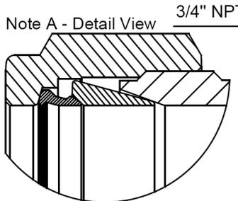
The internal diameter dimension is the minimum nominal opening. These fittings may have a larger opening at the pipe/straight thread end.
