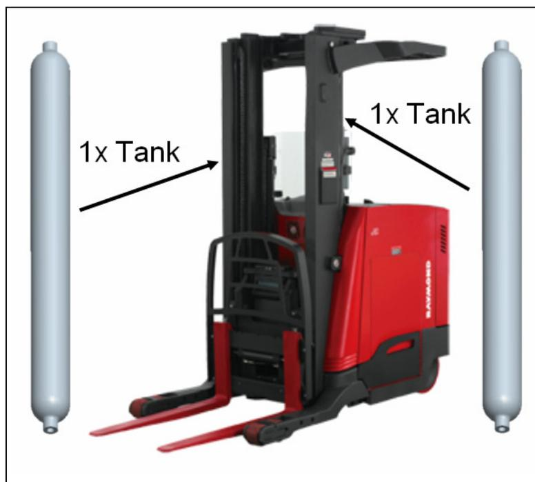
Figure 8 – Mast-Mounted Traditional Cylindrical Vessel
