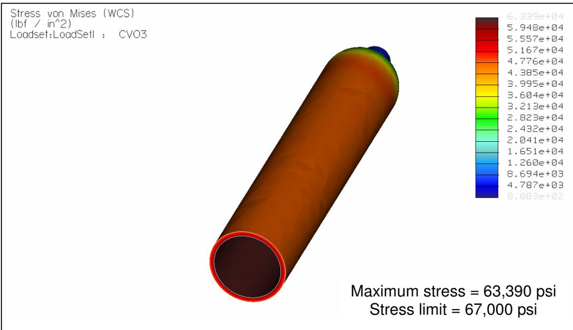
**A-H Figure 8 – 4130 Q&T Cylinder Fringe Plot – Transverse Cut**
