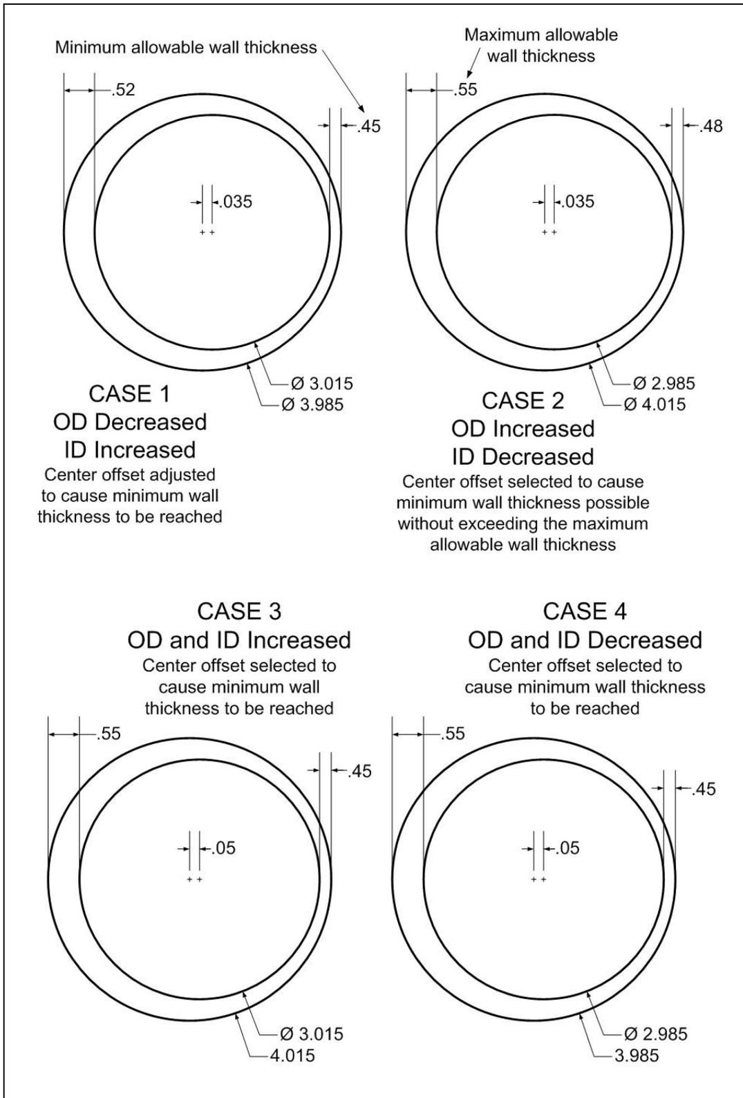
Figure 16 – Maximum Dimensional Variations in 316L Cylinder Tubing
