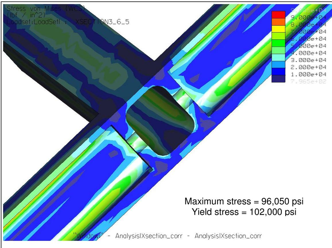
**A-J Figure 33 – 4130 Q&T Hydrostatic X-Section Fringe Plot**
