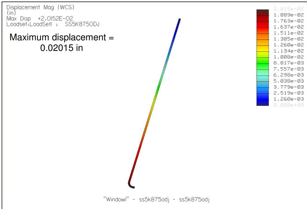
**A-I Figure 14 – 0.875” OD Tube Displacement**
