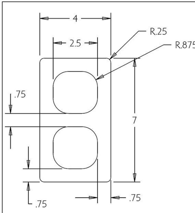
**Figure 28 – 316L SS Cross-Section Design**
