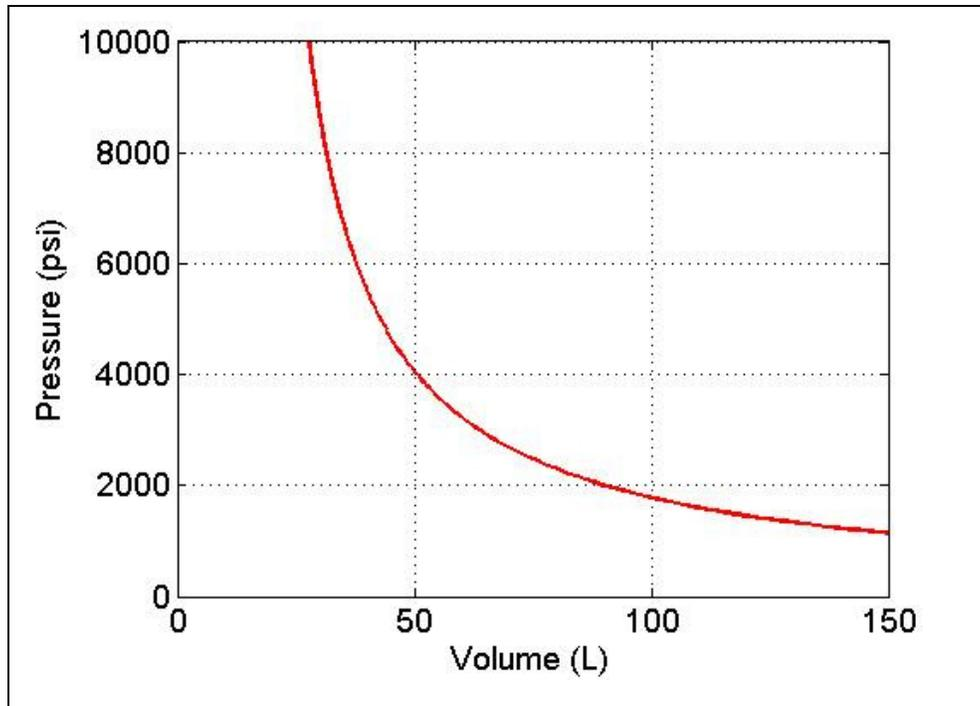
Figure 4 - Pressure vs Volume for Tank Containing 1kg of H<sub>2</sub> at 0°C
