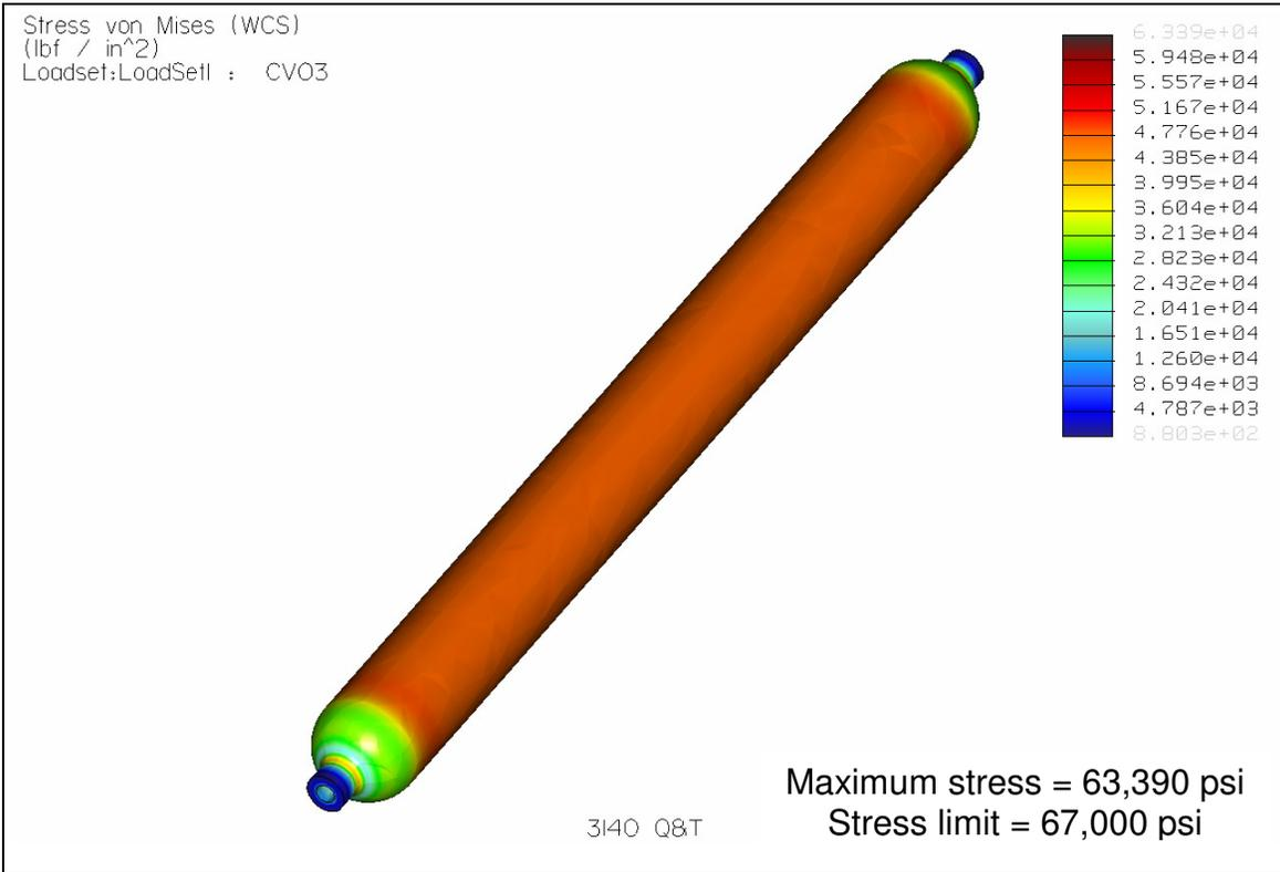
**A-H Figure 7 – 4130 Q&T Cylinder Fringe Plot**
