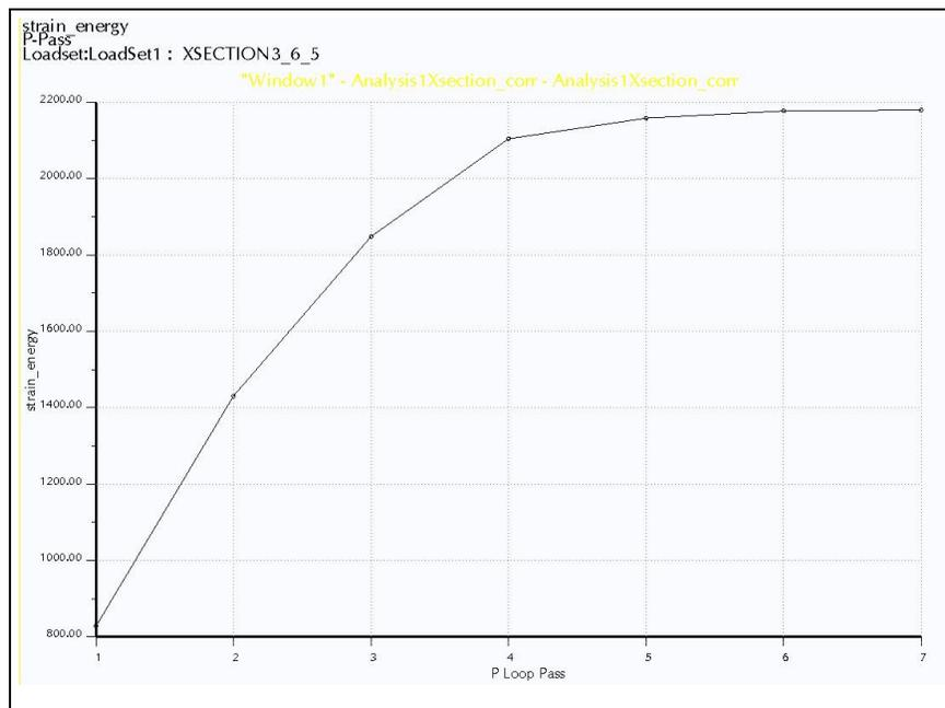
**A-J Figure 34 – 4130 Q&T Hydrostatic X-Section 10% Convergence Plot**
