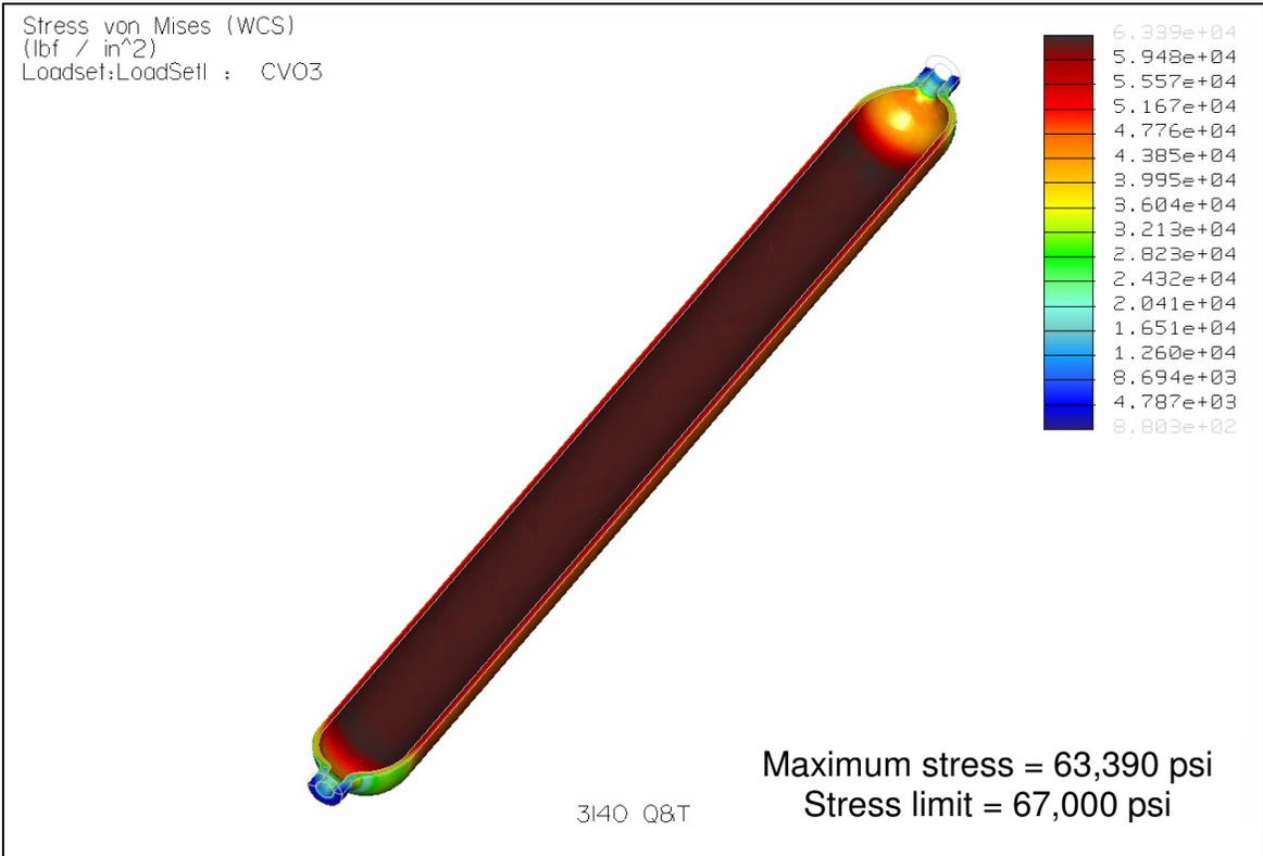
A-H Figure 10 – 4130 Q&T Cylinder Fringe Plot – Longitudinal Cut
