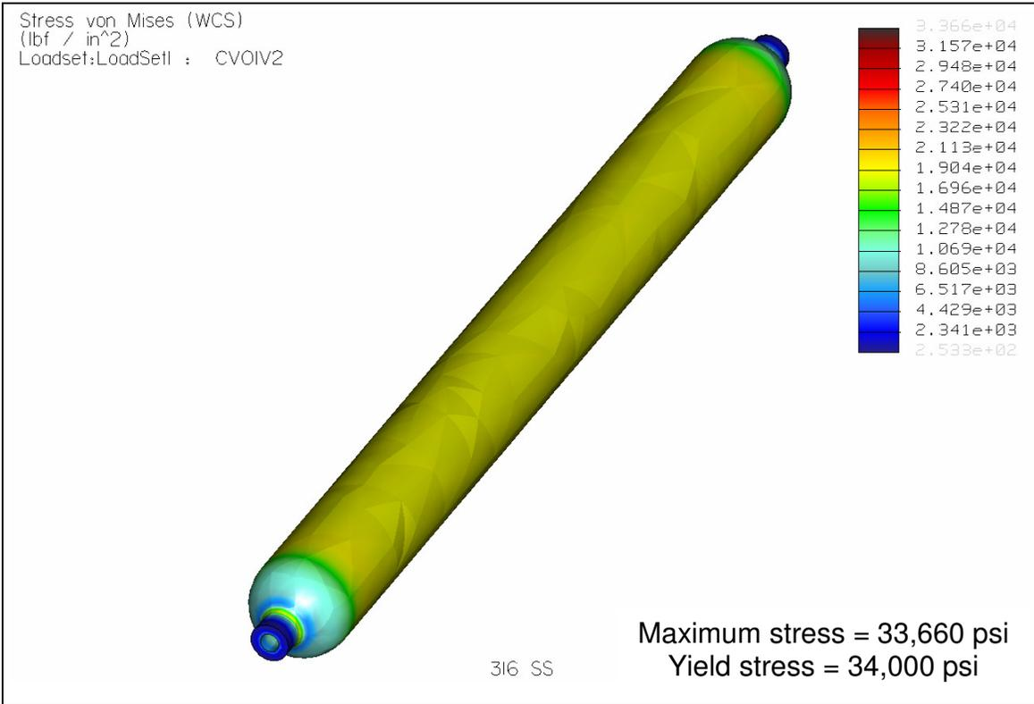
**A-H Figure 1 – 316L SS Cylinder Fringe Plot**
