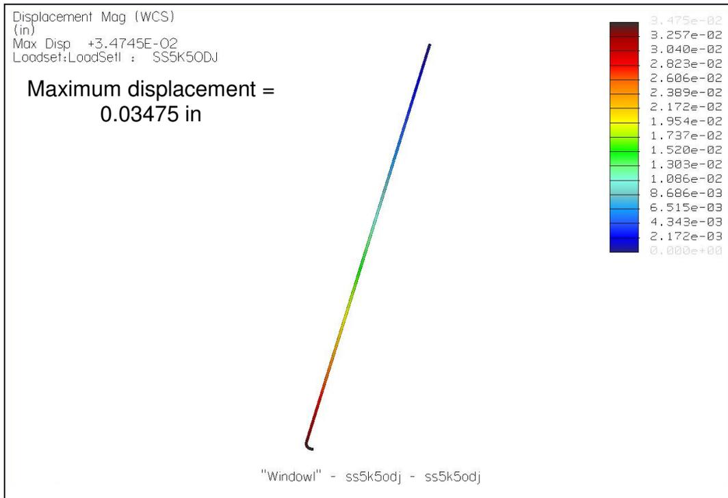
**A-I Figure 16 – 0.5” OD Tube Displacement**
