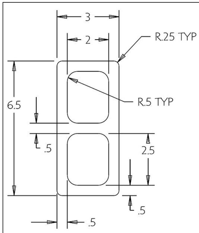
**Figure 31 – 4130 Q&T Cross-Section Design**
