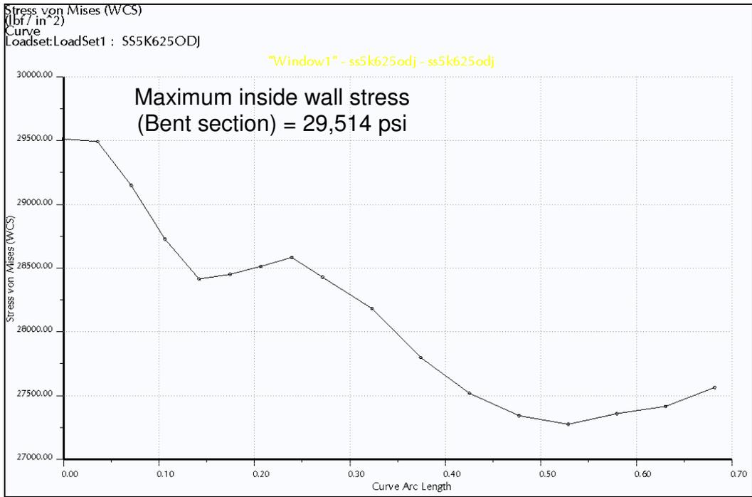
A-I Figure 11 – Stress vs Arc Length (Inside Rim of Bent End, 0.625” OD)
