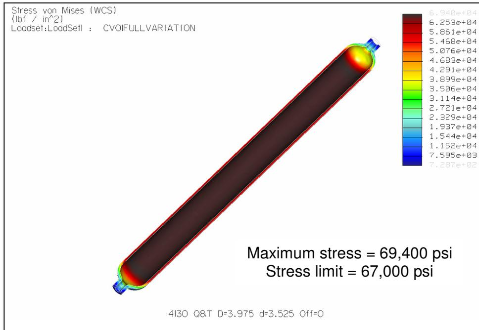
**Figure 18 – 4130 Q&T Cylinder Fringe Plot – Case 1 Variation**
