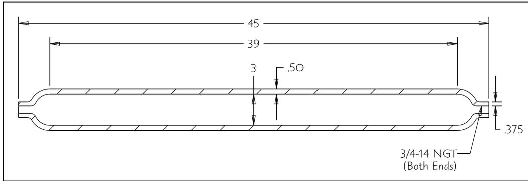
**Figure 11 – Revised Computer Model of 316 SS Cylinder**
