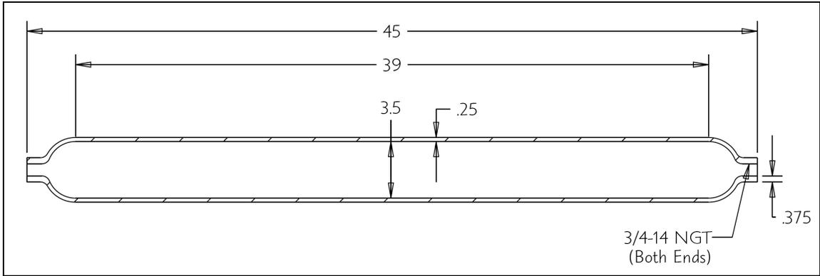
**Figure 13 – Computer Model of 4130 Q&T Cylinder**
