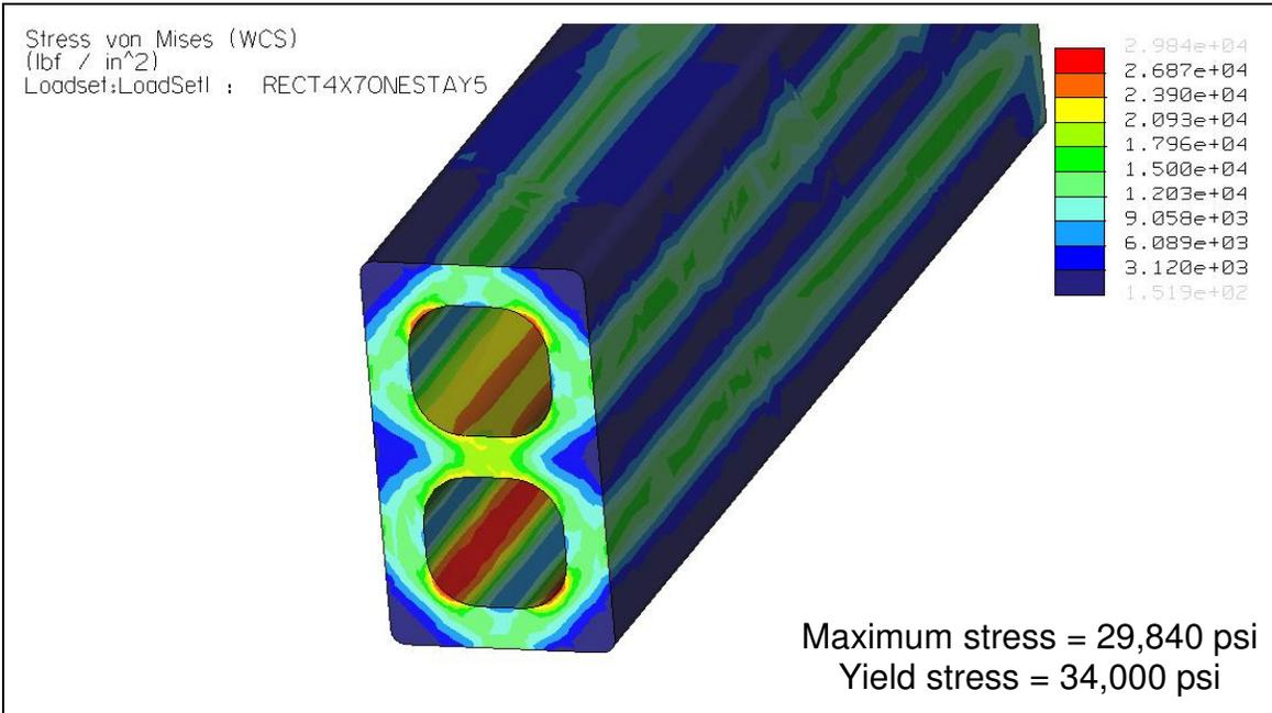
**Figure 27 – 316L SS Straight Section Fringe Plot**
