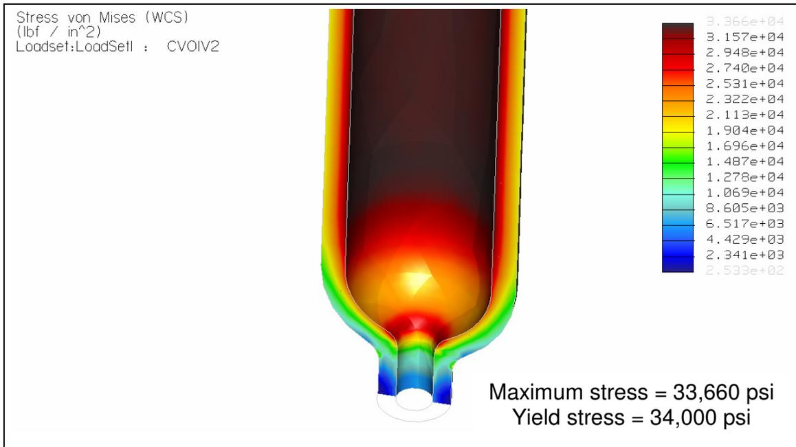
**Figure 12 – 316L SS Cylinder Fringe Plot – Longitudinal Cut Close-Up**
