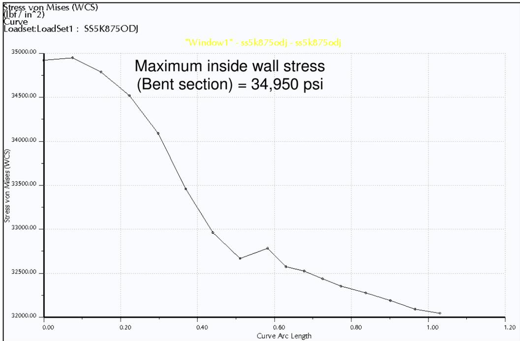
A-I Figure 10 – Stress vs Arc Length (Inside Rim of Bent End, 0.875” OD)
