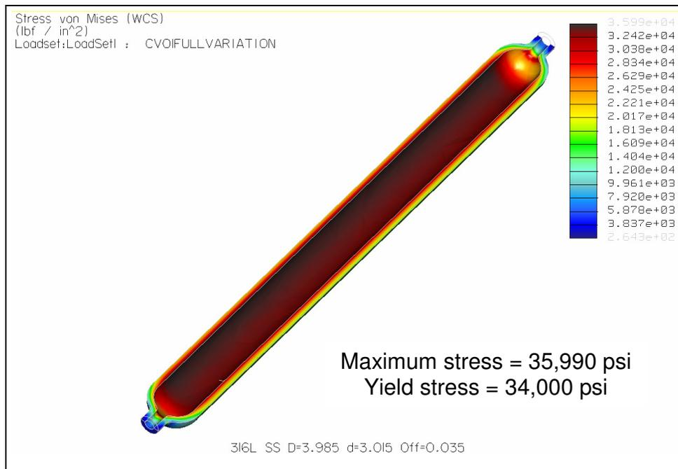
**Figure 17 – 316L SS Cylinder Fringe Plot – Case 1 Variation**
