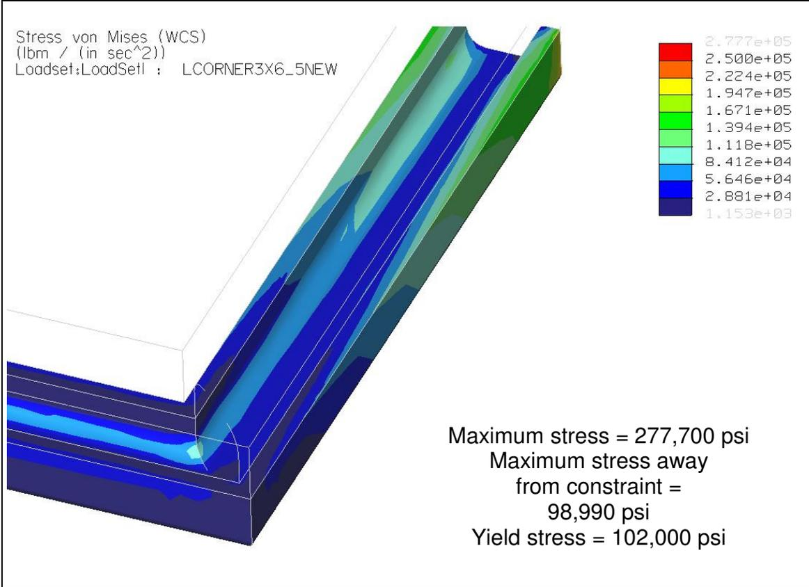
A-J Figure 29 – 4130 Q&T Hydrostatic L-Section Fringe Plot
