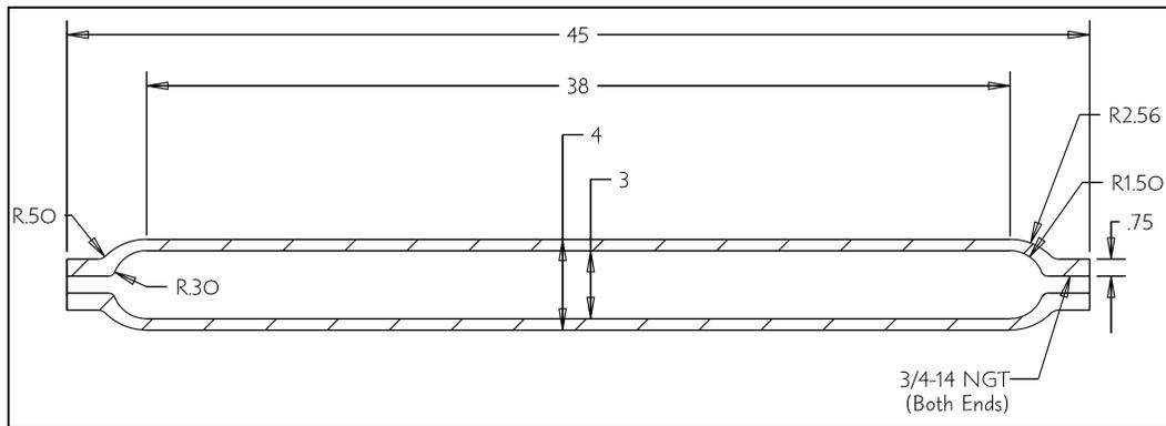
**Figure 10 – First Computer Model of 316L SS Cylinder**
