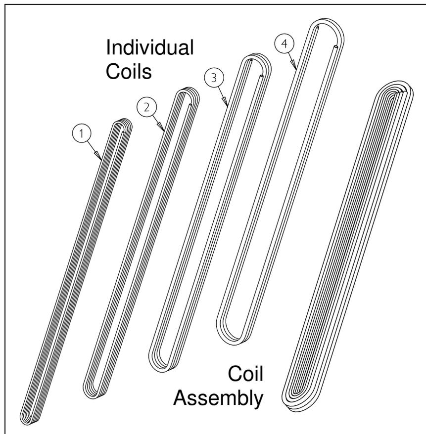
Figure 20 – Coil Configuration
