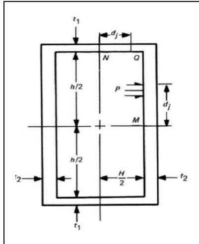
**Figure 25 – Example of Unreinforced Construction**
