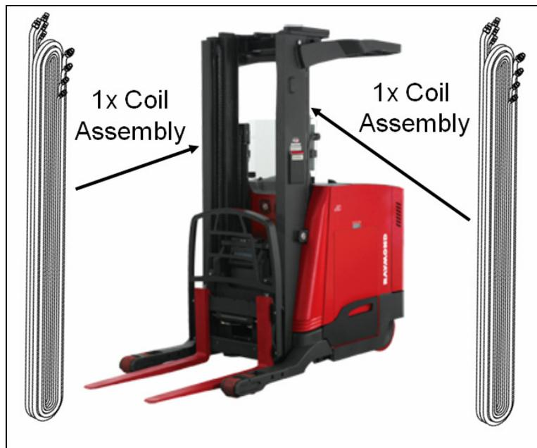
Figure 19 – Mast-Mounted Nested High Pressure Tubing Coils
