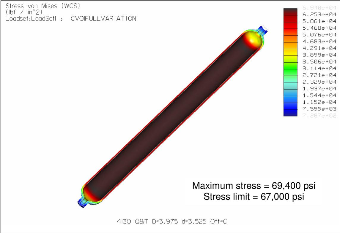
A-H Figure 17 – 4130 Q&T Cylinder Fringe Plot – Case 1 Variation
