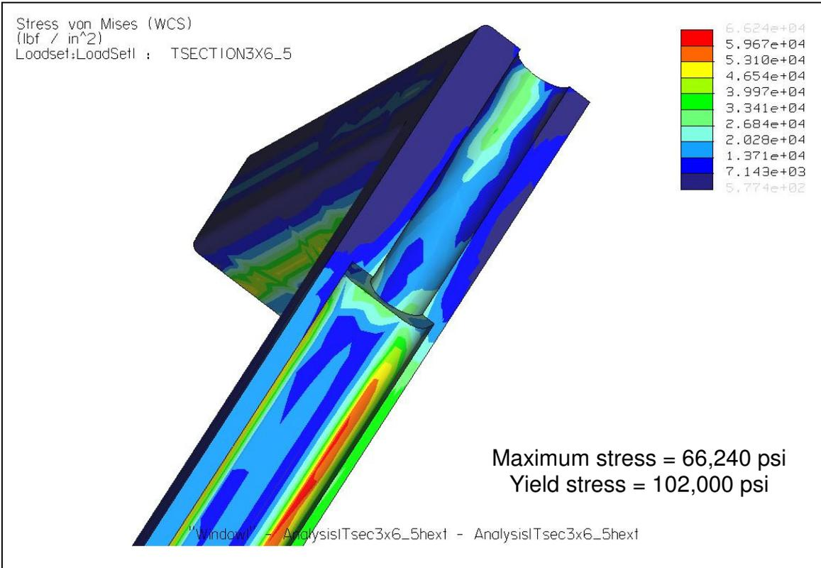
**A-J Figure 13 – 4130 Q&T T-Junction Valve Block Fringe Plot**
