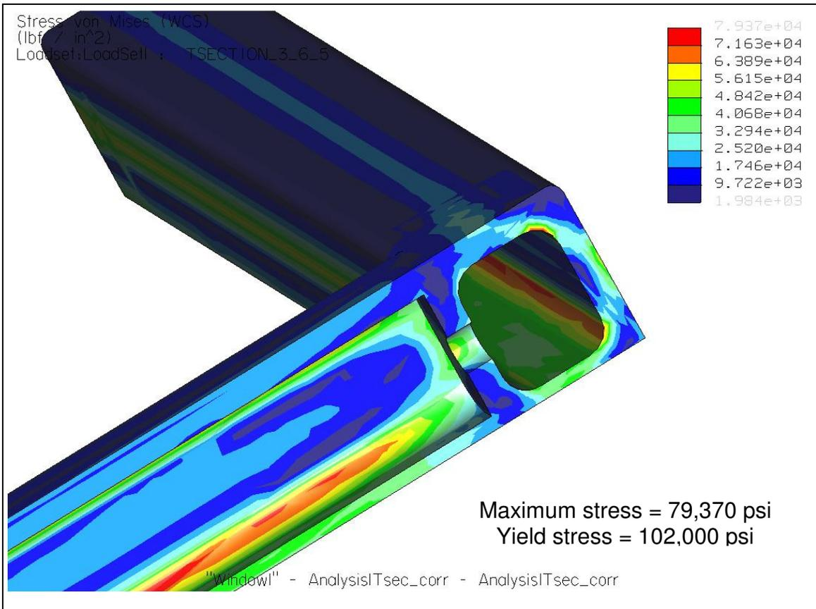
**A-J Figure 31 – 4130 Q&T Hydrostatic T-Section Fringe Plot**
