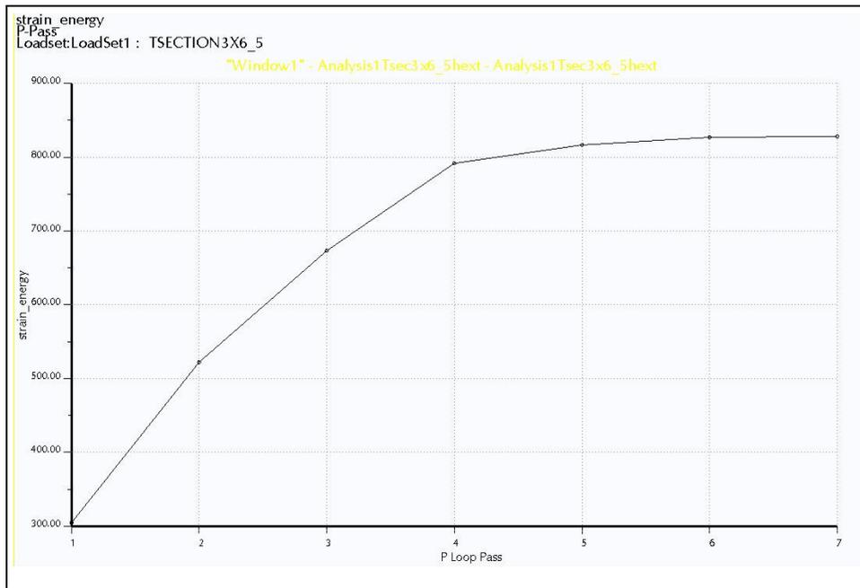
**A-J Figure 14 – 4130 Q&T T-Junction Valve Block 10% Convergence Plot**
