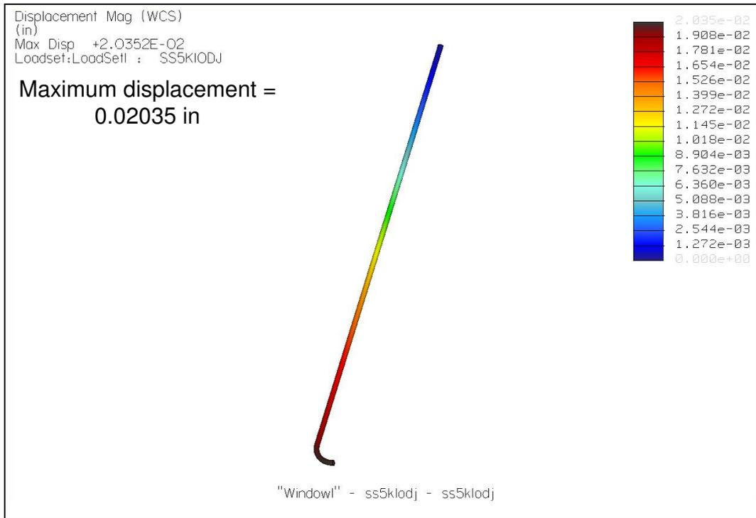
**A-I Figure 13 – 1” OD Tube Displacement**
