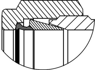
The internal diameter dimension is the minimum nominal opening. These fittings may have a larger opening at the pipe/straight thread end.
