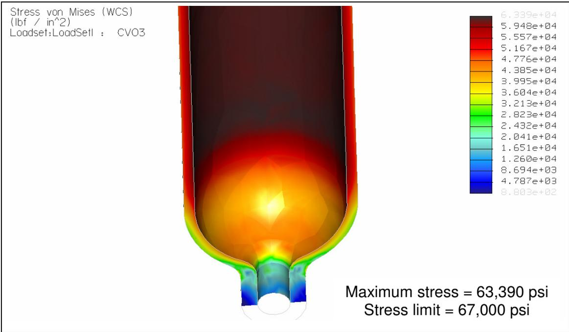
**Figure 14 – 4130 Q&T Cylinder Fringe Plot – Longitudinal Cut Close-Up**
