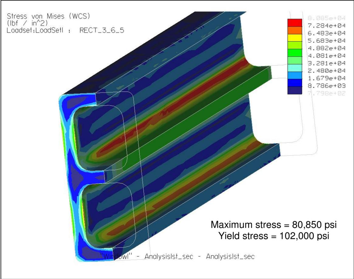
**A-J Figure 27 – 4130 Q&T Hydrostatic Straight Sect Fringe Plot**
