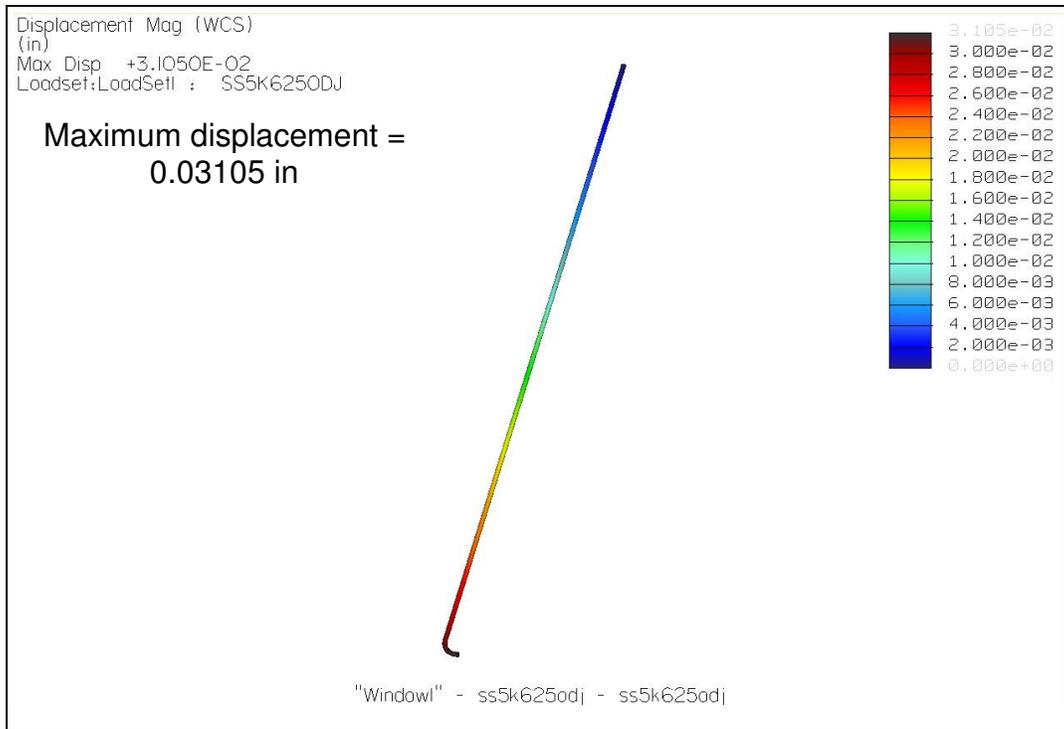
**A-I Figure 15 – 0.625” OD Tube Displacement**
