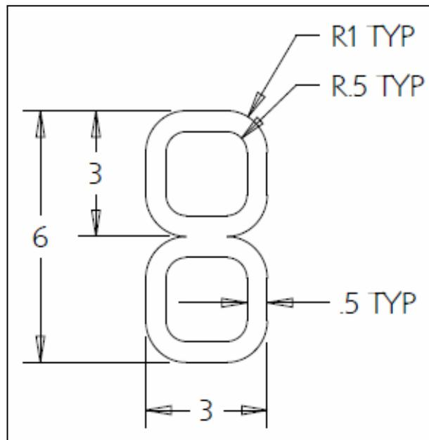
Figure 33 – 4130 Q&T Boxes v1 Cross-Section
