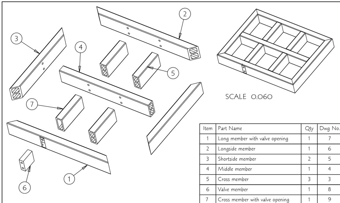
**Figure 32 – 4130 Q&T Assembly Design**
