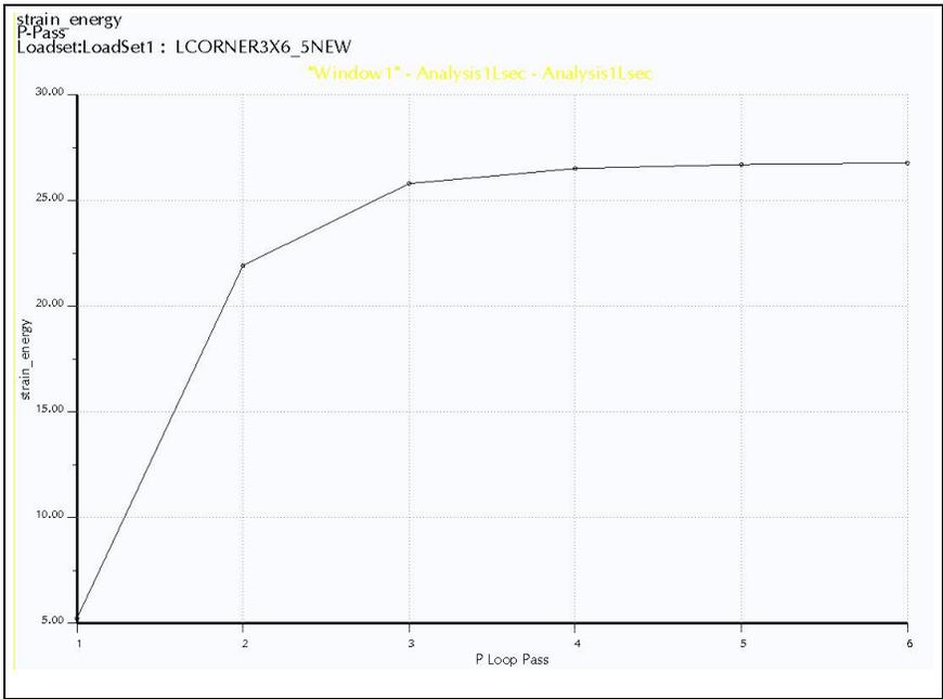
A-J Figure 30 – 4130 Q&T Hydrostatic L-Section 10% Convergence Plot
