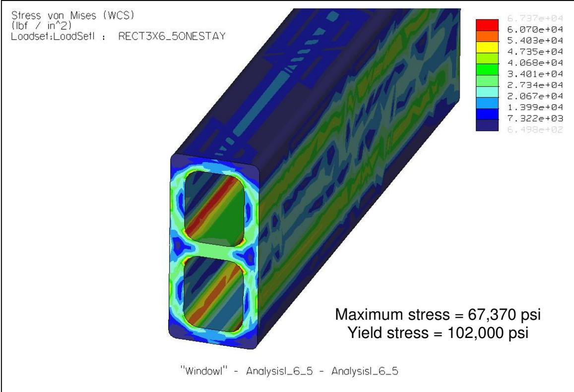
**Figure 30 – 4130 Q&T Straight Section Fringe Plot**
