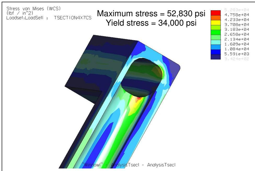
**Figure 29 – 316L SS T-Junction Fringe Plot**
