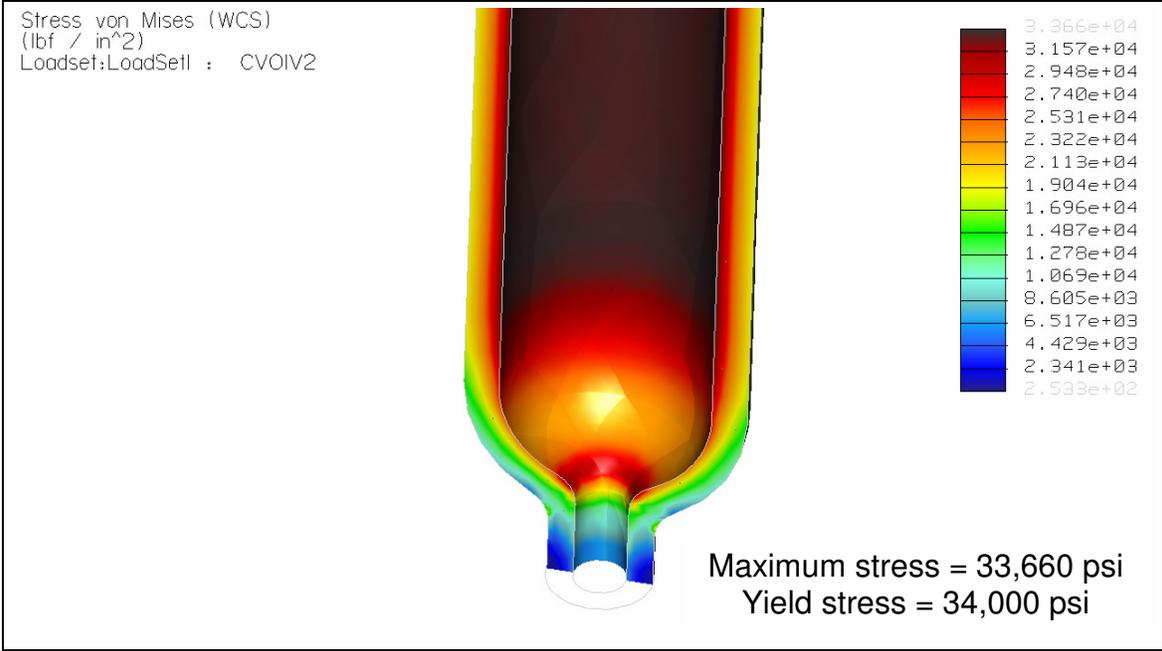
**A-H Figure 5 – 316L SS Cylinder Fringe Plot – Longitudinal Cut Close-Up**
