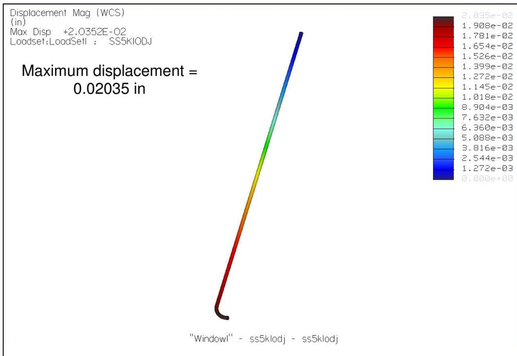
**Figure 22 – 1” OD Tube Displacement**
