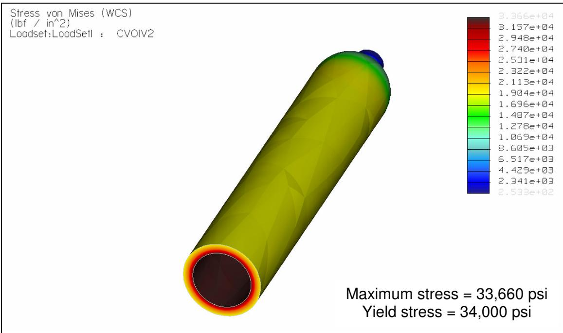
**A-H Figure 2 – 316L SS Cylinder Fringe Plot – Transverse Cut**
